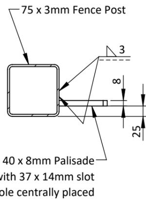
M12 x 40 Coach Bolt with Shear Nut fixed to Welded Tab
